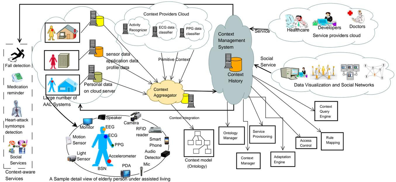
Fig. 1. **The Generic Model:** Data generated in AAL systems converted to context model in *Context Aggregator* with the help of various *Context Providers*. *CMS* manages context from users and service from *Service Providers* and associates context-aware services. Different modules runs inside *CMS* as cloud service
